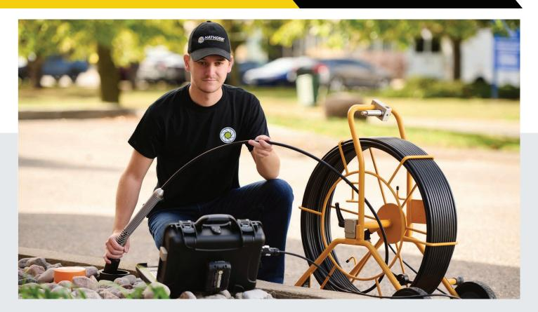
Hathorn® camera reels are designed to work with any Hathorn control module, past present or future. These rugged and durable camera reels come fitted with your choice of Hathorn self-levelling camera heads, all equipped with super-bright, cool running LEDs for optimal picture quality.
